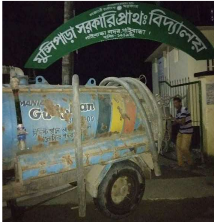
(a) Cleaning preparation of septic tank by using vaccu-truck at Gaibandha
